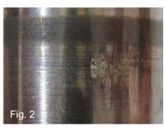
Current passage has led to a formation of craters/flutes on the inner ring raceway (fig. 1) and the lateral surface of the rolling elements (fig. 2) of a cylindrical roller bearing
